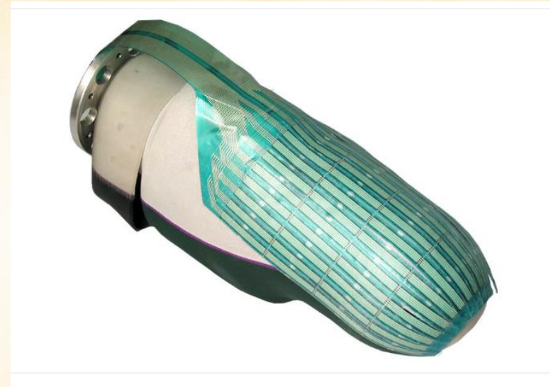
F-Socket Software provides information on peak pressures, force vs. time graphs and center of force (CoF).
